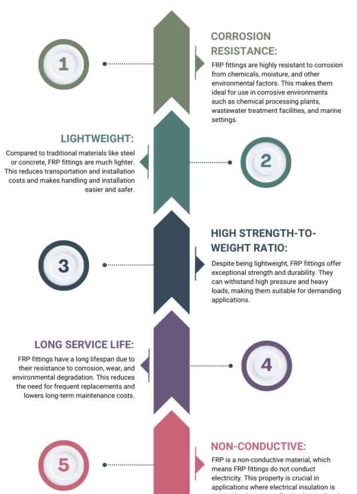
required, enhancing safety in electrical and electronic installations.
